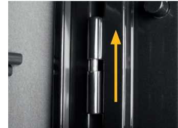
Illustration 1. The door must be clear of its frame before it can be removed. Lift it straight up so as not to damage the bolts.
